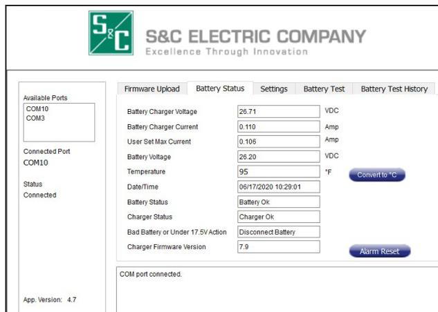
Figure 5. The *Battery Status* screen.
