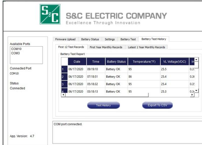
Figure 11. The **Battery Test History** screen.
