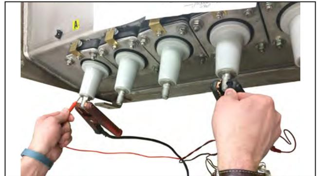
**Figure 56. Connecting the resistance measuring device.●**
