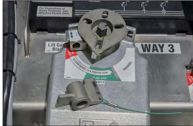
Figure 16. The operation selector in the far left position.
