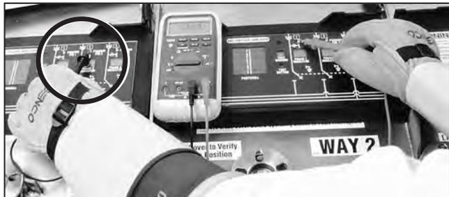
**Figure 51. Measuring the phase-to-phase voltage—Phase 2 to Phase 1**
