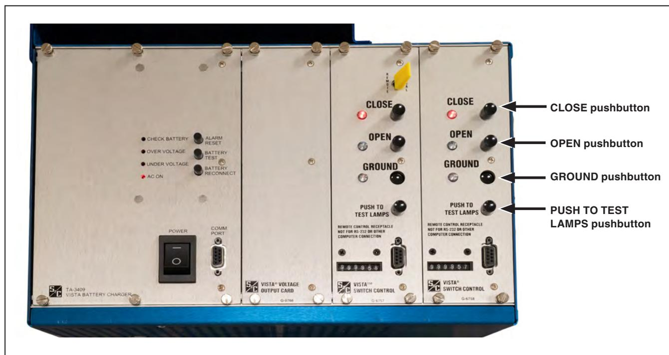
Figure 34. The motor operator control board pushbuttons.
