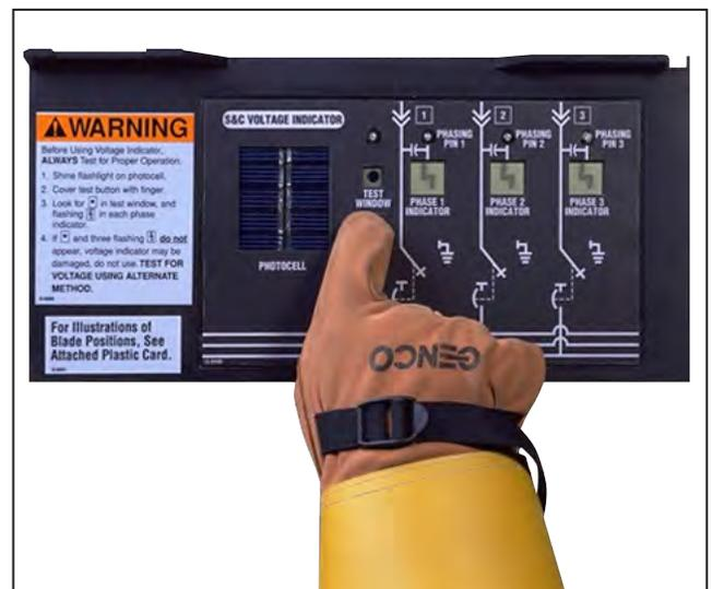
Figure 44. The VOLTAGE indicator is operating properly if a dot appears in TEST window and a flashing lightning bolt appears in each PHASE indicator.
