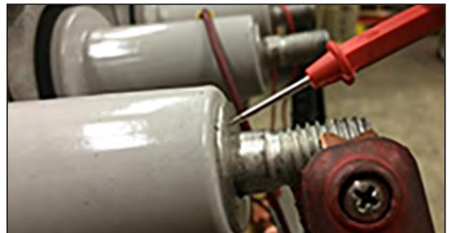
**Figure 57. Take the measurement from the flat current-carrying surface of the bushing.●**
