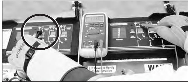
**Figure 50. Measuring the phase-to-phase voltage—Phase 1 to Phase 1**
