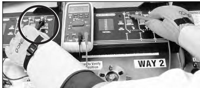
**Figure 52. Measuring the phase-to-phase voltage—Phase 3 to Phase 1**
