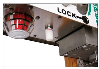
Figure 14. The Wi-Fi antenna is located on the underside of the base.
