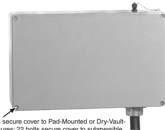
**Four captive screws** secure cover to Pad-Mounted or Dry-Vault-Mounted Style enclosures; 22 bolts secure cover to submersible enclosures (tightened to 15 foot-pounds)
