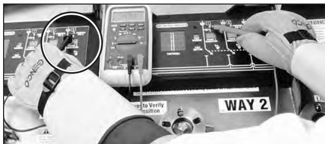
**Figure 55.** Measure the phase-to-phase voltage—Phase 3 to Phase 1.
