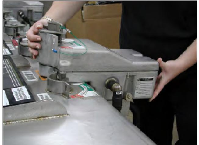
Figure 41. Reposition the motor operator.
