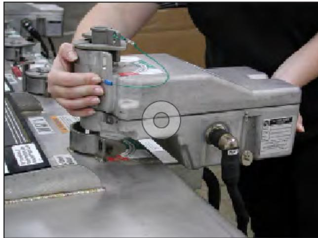
Figure 39. Lift the motor operator.
