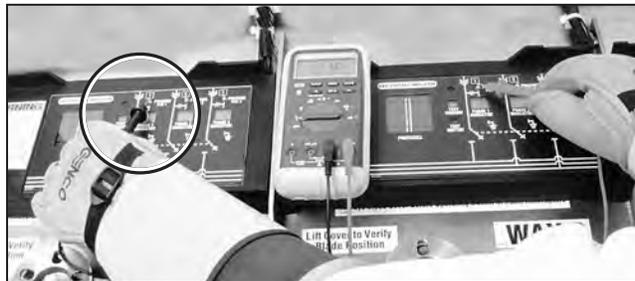
**Figure 53.** Measure the phase-to-phase voltage—Phase 1 to Phase 1.
