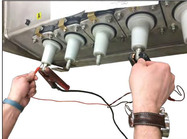
**Figure 60. Connecting the resistance measuring device.●**
