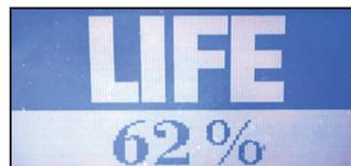
Figure 30. The *Remaining Contact Wear in %* screen.
