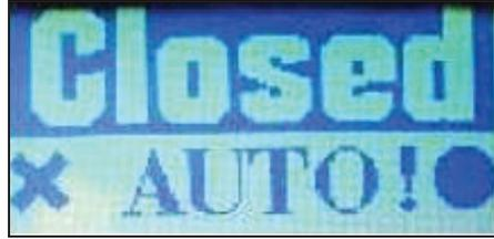
Figure 52. Exclamation point indicator for a battery abnormality.
