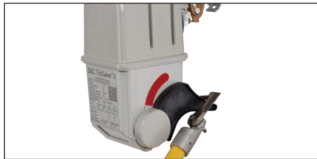
Figure 16. Place the prong above the lever and pull down to enter NR mode.
