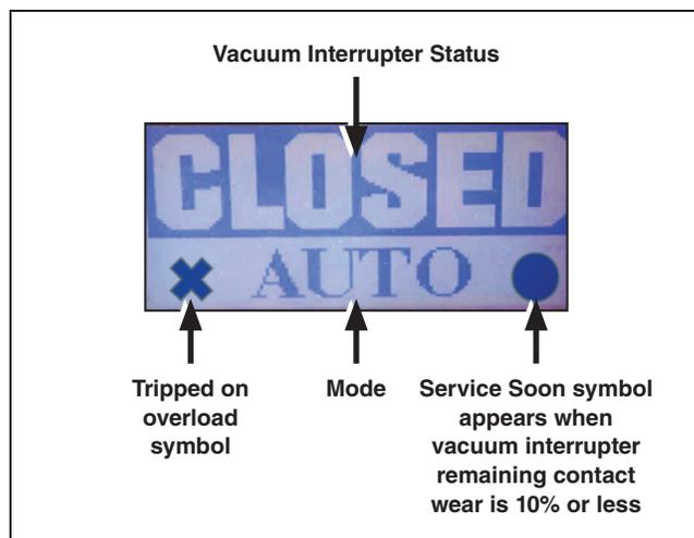
Figure 26. Illustration of the *Primary Normal* screen.
