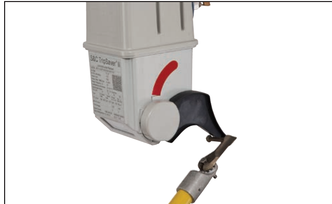
Figure 15. Place the prong under the lever and push up to enter Auto mode.
