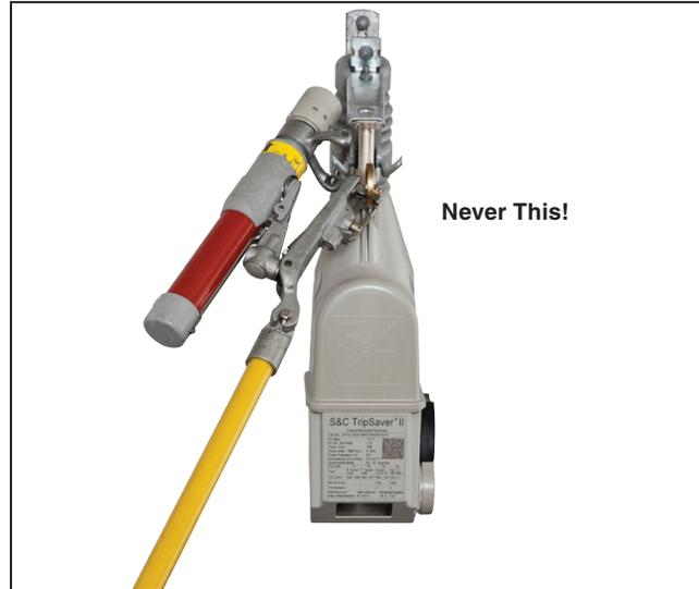
Figure 36. An incorrect fastening approach.
