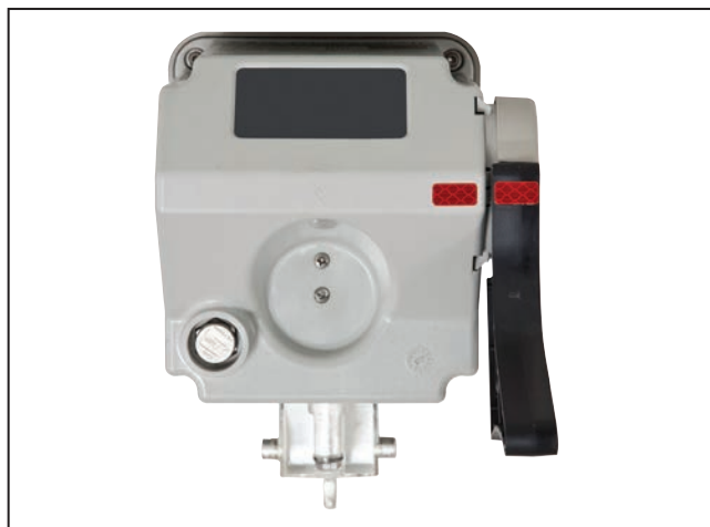
Figure 23. Align the lever with the label on the body.
