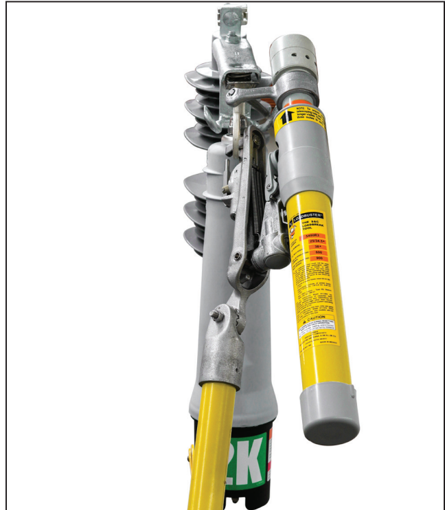
Figure 16. A correct fastening approach.
