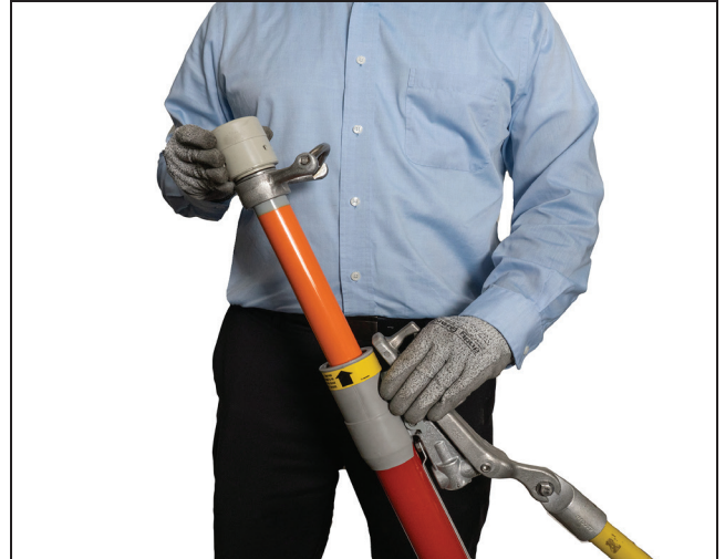
Figure 21. Resetting the Loadbuster tool.
