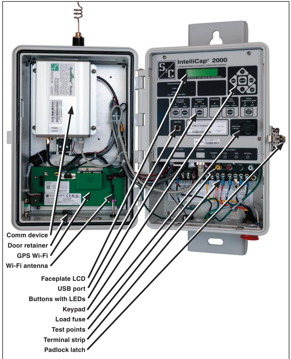
Figure 2. Interior of the IntelliCap 2000 control.
