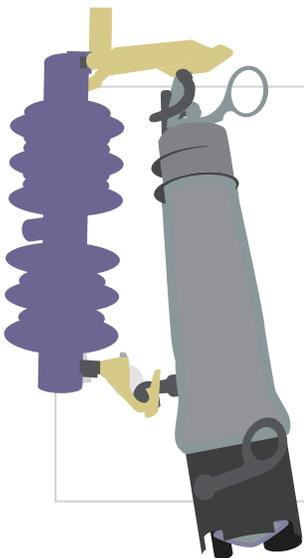
Accompanying the wide range of lateral protection offered by TripSaver II recloser, the VacuFuse II Self-Resetting Interrupter provides grid-edge protection for customers in the most vulnerable locations on your system.
