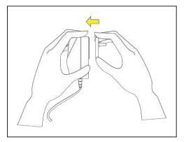
Figure 14. Installing the outlet plug adapter.
