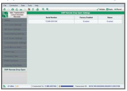
Figure 139. The DNP Remote Drop Open screen, when connected via the USB transceiver.
