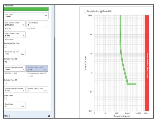
Figure 80. Example of a 100ST fuse curve with one definite time
