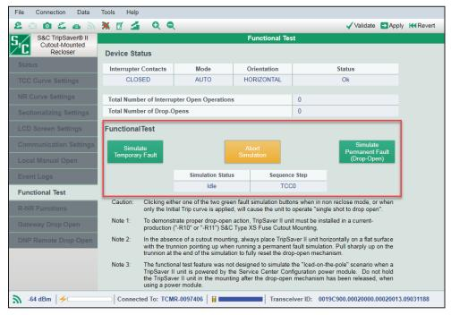
Figure 123. The Functional Test command area.
