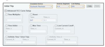
Figure 91. The Advanced TCC Curve Setup when Hydraulic Recloser is selected under Emulated Device.
