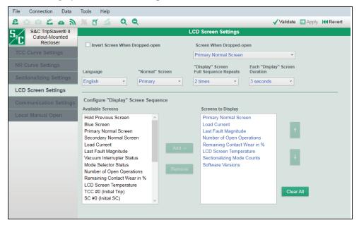
Figure 98. The LCD Screen Settings screen.
