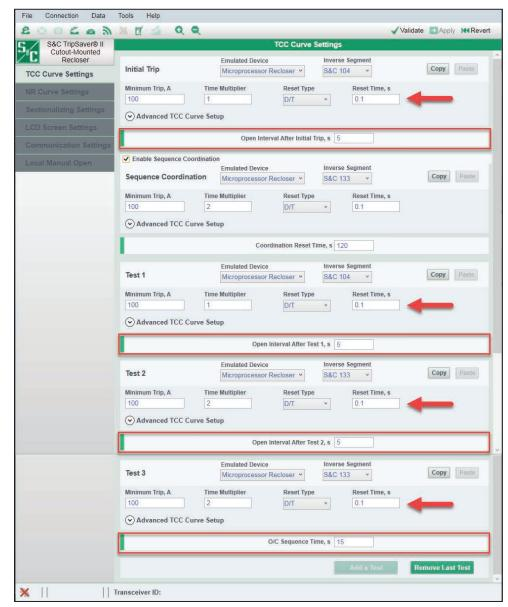
Figure 67. The Open Interval and O/C Sequence Time setting field locations.
