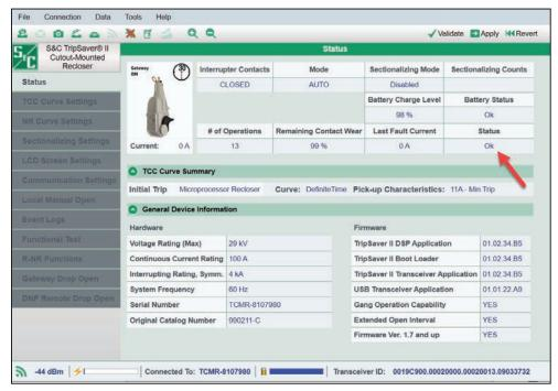
Figure 151. The Status screen after a successful Clear Service Now reset procedure.
