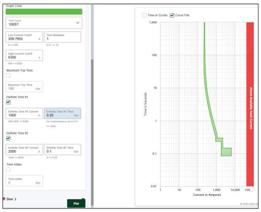
Figure 81. Example of a 100ST fuse TCC curve with two definite times.
