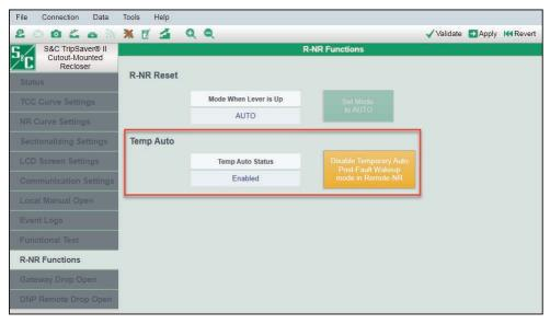
Figure 136. Enable or disable Temporary Auto mode when the recloser is in R-NR mode.
