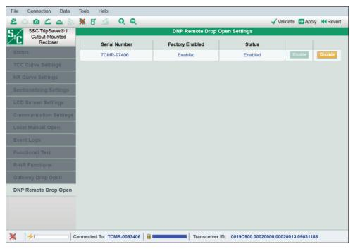
Figure 140. The DNP Remote Drop Open screen, when connected via the communication gateway.
