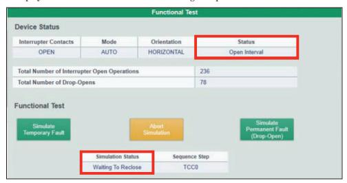
Figure 124. The status during functional test open interval.
