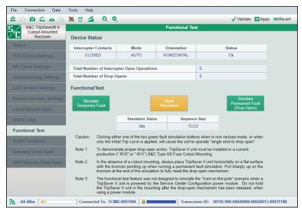
Figure 121. The Functional Test screen.
