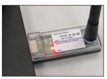
Figure 142. LED indicators on the USB Transceiver.
