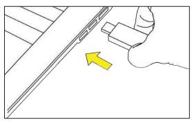
Figure 11. Inserting the USB transceiver into the computer.
