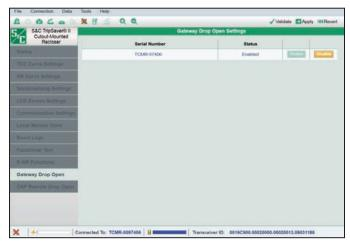
Figure 138. The Gateway Drop Open Settings screen, when connected via communications gateway.
