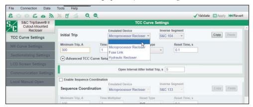
Figure 68. The blank option for clearing the TCC setting.
