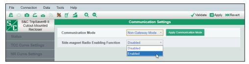
Figure 134. The Side-Magnet Radio Enabling Function option.
