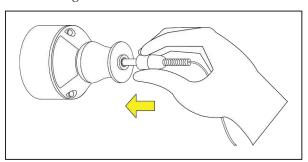
Figure 12. Inserting the power connector into the power module.
