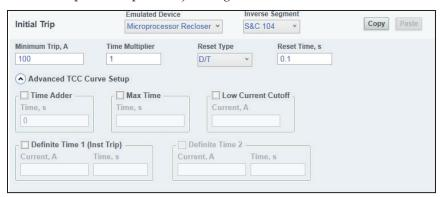
Figure 75. The Advanced TCC Curve Setup fields for a microprocessor recloser.
