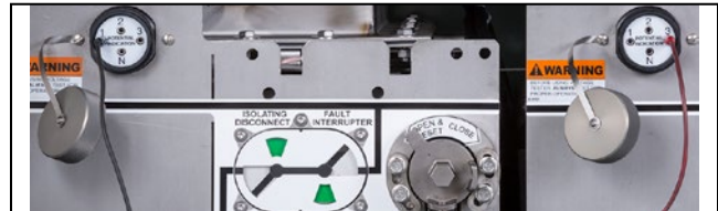
Figure 33. Measure the phase-to-phase voltage between Test Jacks 1, 2 and 3 of the first way and Test Jack 3 of the second way.
