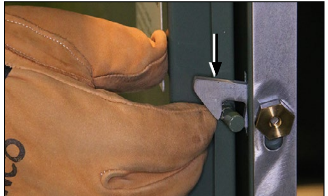
Figure 35. Fully engage the door latch mechanism.
