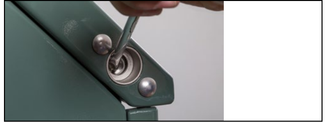
Figure 50. Rotate the actuator with a screwdriver until the latching mechanism closes.
