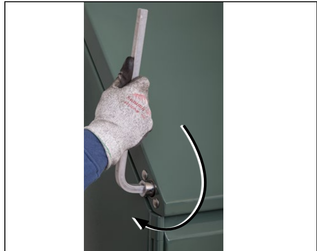
Figure 37. To fully latch the hinged roof, rotate the pentahead socket wrench or tool 360° clockwise. .
