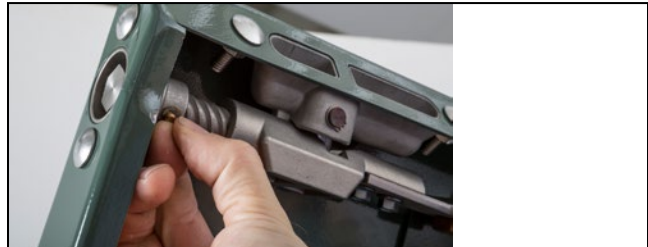
Figure 47. Install a retaining ring on the opposite side of the shear pin.
