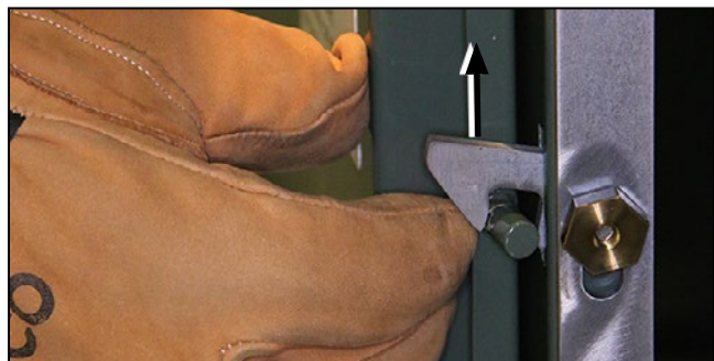
Figure 49. To open the left-side door, lift the finger latch.
