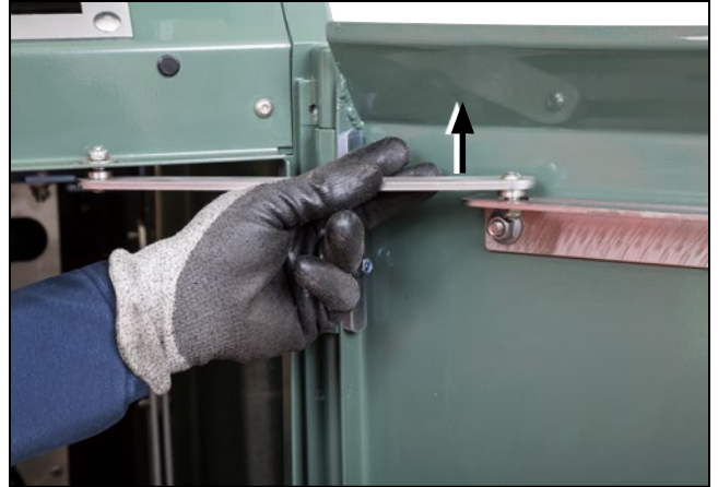
Figure 34. Lift the door-holder mechanism up to allow the door to swing closed.
