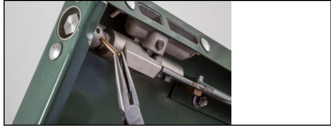
Figure 46. Install the new shear pin.
