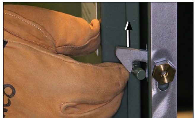
Figure 11. To open the left-side door, lift the finger latch.
