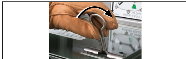
Figure 13. Rotate the operating handle guide ring to the active (Up) position.
