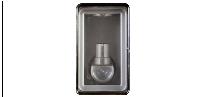
Figure 23. The isolating disconnect after the fault interrupter has been opened and reset.
