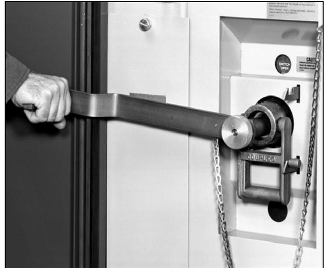
**Figure 18.** Dual-purpose manual handle reverse-driving the Mini-Rupter Switch and operator's quick-make quick-break mechanism to recover from a stalled condition.
