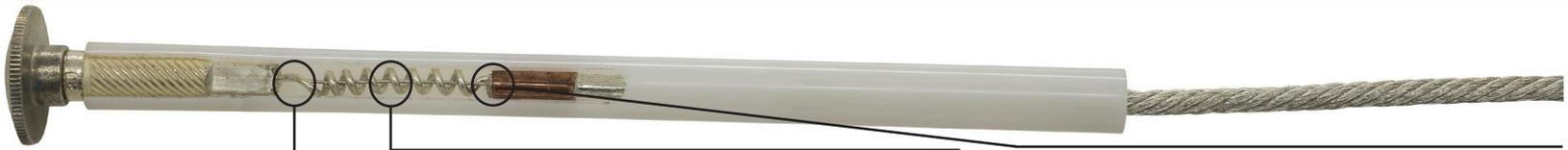
**Silver Elements** - Silver melts at a higher temperature. During 90% of its melting time, silver is in the heating phase and absorbs a lot of heat before melting. This allows fuse links with silver\* elements to carry currents very close to the minimum melting time without any damage to the element itself.
