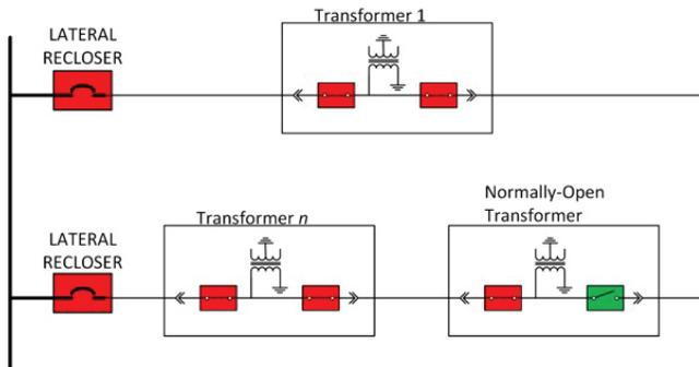
Figure 4. Future State of Underground Lateral with Automation
