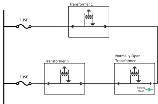
Figure 3: Typical Underground Residential Distribution Lateral
