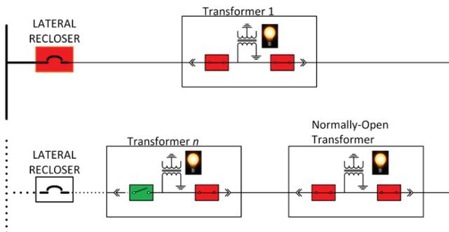
Figure 7: Loss of Voltage Case 2 – after restoration
