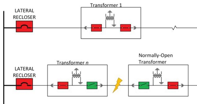
Figure 5. Isolation of a Faulted Segment
