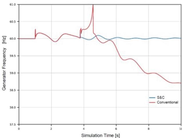
Figure 5. Generator frequency response using LEI technology (blue curve) vs. conventional reclosing technology (red curve) following a close-in permanent fault.
