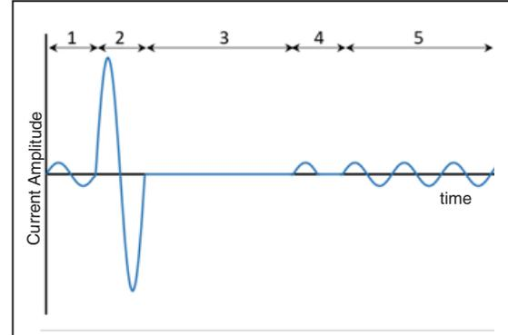
Figure 2. Low-Energy Testing after detecting and interrupting a temporary fault.
