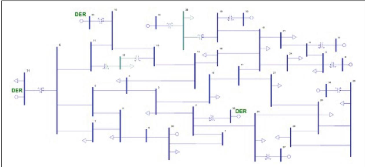
Figure 3. One-line diagram of the modified IEEE 39-Bus system model with 20% DER penetration indicating location of the N-1 contingency.
