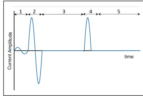
Figure 1. Low-Energy Testing after detecting and interrupting a permanent fault.
