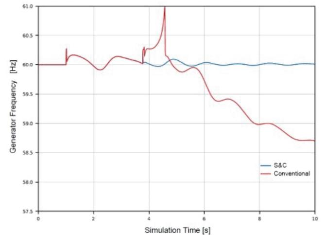
Figure 7. Generator frequency response using LET technology (blue curve) vs. conventional reclosing technology (red curve) following a close-in permanent fault.
