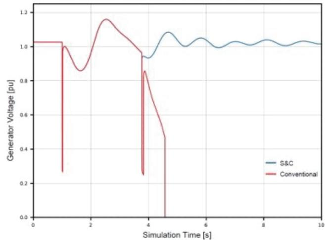
Figure 6. Generator voltage response using LET technology (blue curve) vs. conventional reclosing technology (red curve) following a close-in permanent fault.
