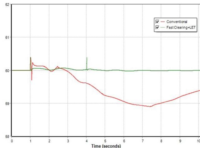
Figure 9. System frequency response following a temporary fault using LEI/LET technology compared to conventional reclosing.
