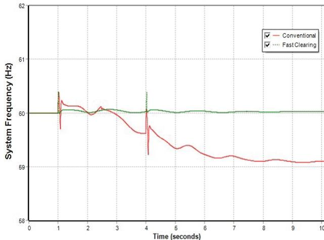
Figure 8. System frequency response following a permanent fault using LEI/LET technology compared to conventional reclosing.
