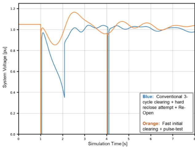
Figure 4. Generator voltage response using LEI/LET (orange curve) vs. conventional clearing (blue curve) following a close-in permanent fault.
