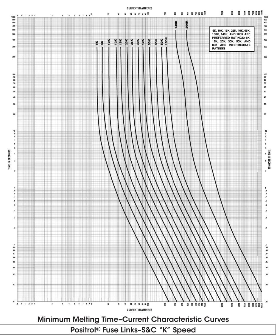
BASIS-These fuse links are tested in accordance with the procedures described in IEEE Standard C37.41, to comply with IEEE Standard C37.42. As required by these standards, the minimum melting current is not less than 200% of fuse-link ampere rating, and the minimum melting curves are based on tests starting with the fuse link at an ambient temperature
