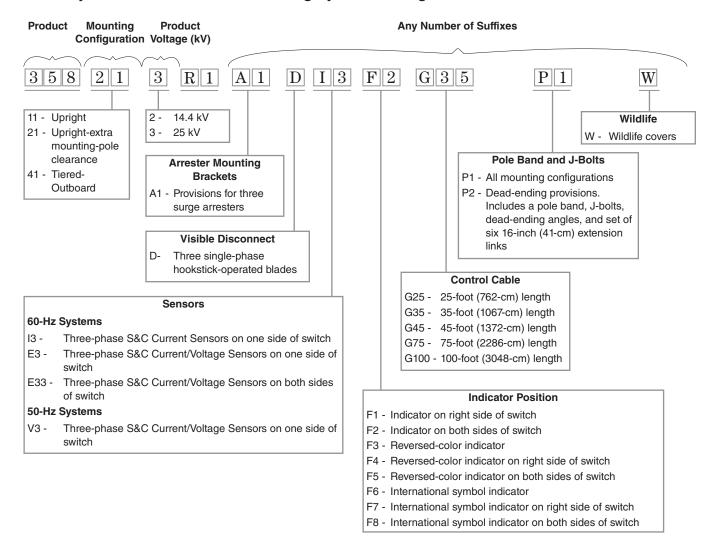
The catalog number created above represents a 25-kV upright-extra mounting-pole clearance Scada-Mate SD switch. It comes with three arrester brackets for one side the switch, a manual disconnect, and wildlife protection. It also comes with a 60-Hz current sensor and voltage sensors on each side of the switch. To connect to the control unit, a 35-foot (10.7-m) cable option is chosen. A pole band and J-bolts are included.
