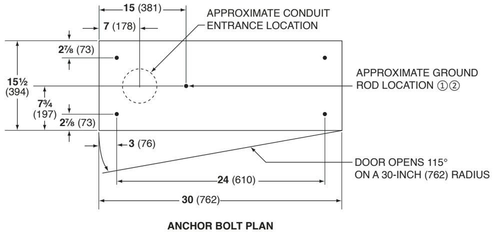
① Attach earth ground cable between the ground lug inside the low-voltage enclosure and the ground rod using copper cable of 4/0 or greater and less than 10 feet (305 cm) in length.
