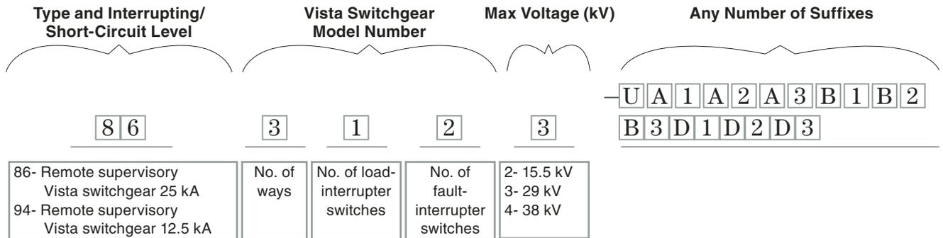
**Note:** The catalog number created above represents an UnderCover™ Style remote supervisory Vista switchgear unit, 25 kA, with a total of three ways that includes one load-interrupter switch and two fault-interrupter switches for a 29-kV application. All three ways will have the motor operator package, three-phase current sensing, and three-phase voltage sensing.
