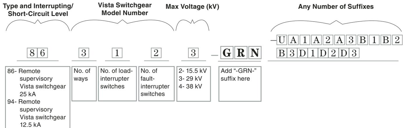
**Note:** The catalog number created above represents an UnderCover Style remote supervisory Vista Green switchgear (CO<sub>2</sub> mix) unit, 25 kA, with a total of three ways that includes one load-interrupter switch and two fault-interrupter switches for a 29-kV application. All three ways will have the motor operator package, three-phase current sensing, and three-phase voltage sensing.
