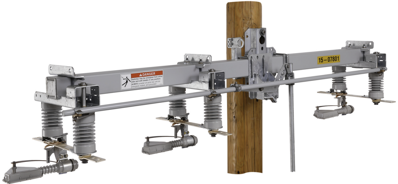
Figure 1. 14.4-kV reciprocating operating handle Omni-Rupter Switch in the inverted mounting configuration.
