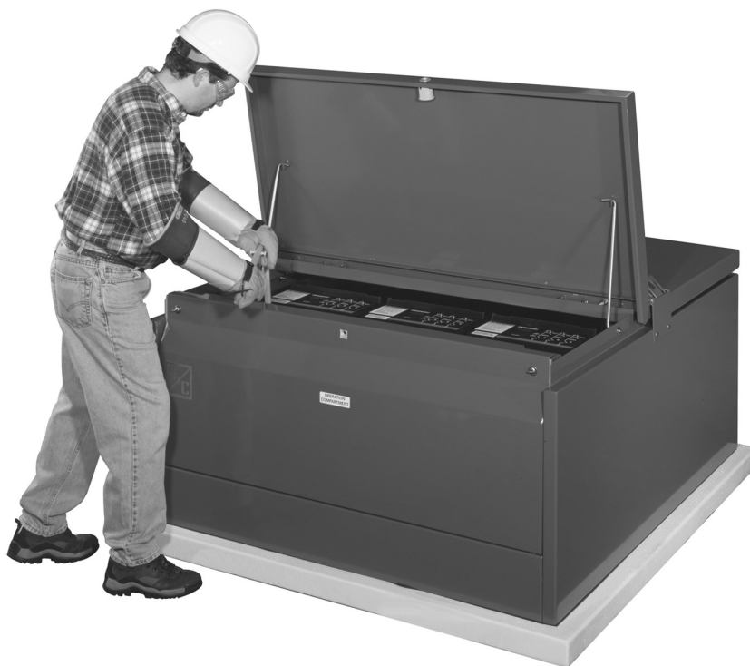
The 15-kV pad-mounted models provide more space for cable accessories such as feed-thru inserts, surge arresters, and piggy-backed T-bodies.
