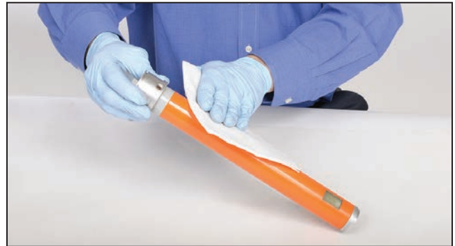
Figure 30. Apply a layer of silicone oil.
