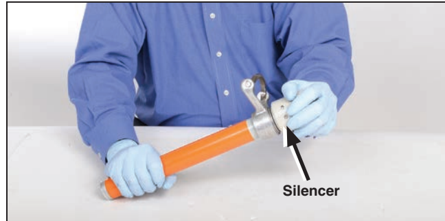
Figure 8. Remove the silencer.
