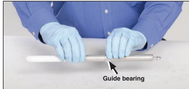
Figure 40. Install the guide bearing.
