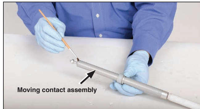
Figure 41. Apply lubricant to the trigger end of the moving contact assembly.
