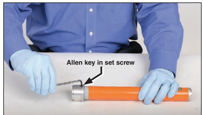
Figure 12. Remove and discard the set screw.
