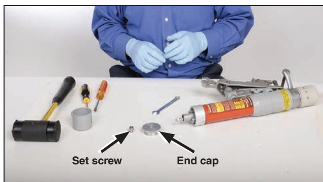
Figure 4. Remove the set and retaining screws.
