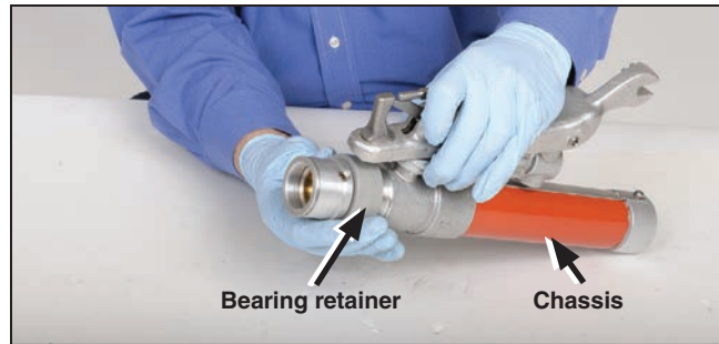
Figure 33. Thread the bearing retainer onto the chassis.
