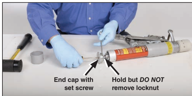
Figure 3. Hold the locknut steady and loosen and remove the set screw.
