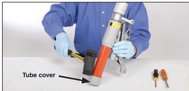
Figure 1. Use a mallet to loosen the tube cover.
