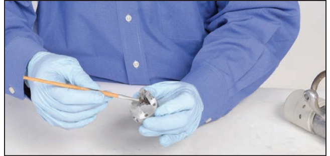
Figure 43. Apply lubricant to the latching area of the trigger.
