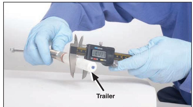
Figure 19. Measure the diameter of the trailer. Do not measure the chamfered ends.
