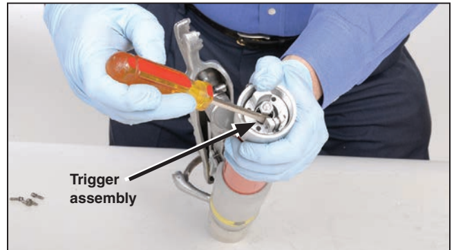
Figure 44. Insert the trigger into the inner tube assembly. Depress the trigger to extend the moving contact assembly.
