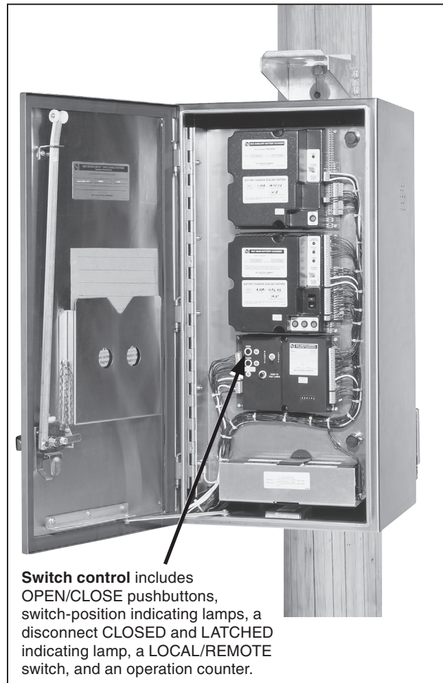
Figure 26. Operating the switch using the LOCAL/REMOTE switch inside the control unit.
