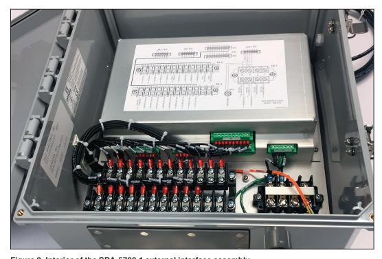
Figure 2. Interior of the SDA-5798-1 external interface assembly.
