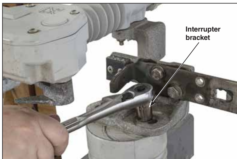
Figure 35. Remove the cap screws and washers securing the interrupter bracket to the insulator.
