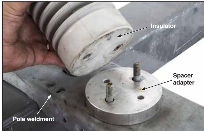
Figure 36. Remove the insulator. Align the spacer adapter with the holes on the pole weldment, with the mounting hole recesses facing down. Align insulator with the mounting holes, and secure with bolts.
