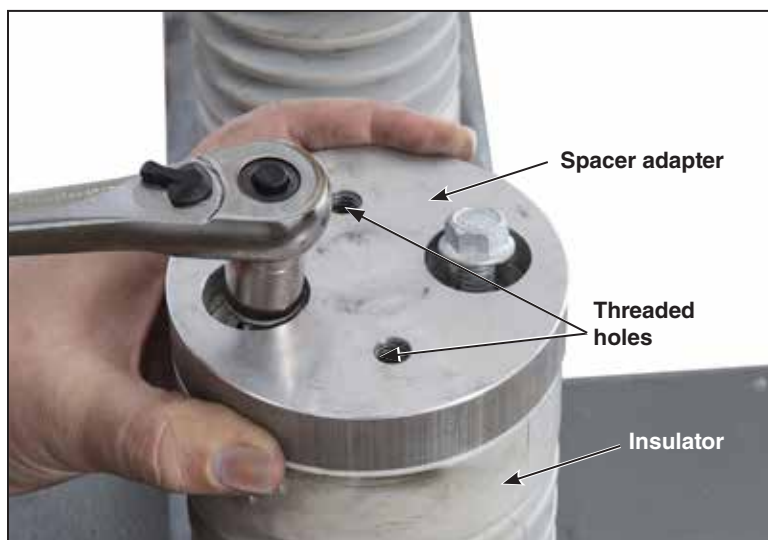
Figure 33. Align the spacer adapter with the holes in the insulator and tighten.
