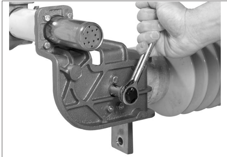
Figure 19. Attaching current-carrying contact assembly.
