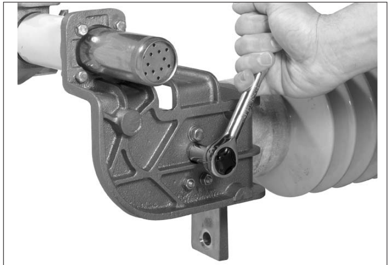
Figure 7. Removing current-carrying contact assembly.
