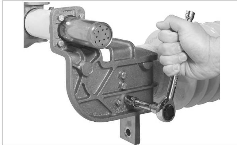
Figure 8. Removing arcing contact assembly.
