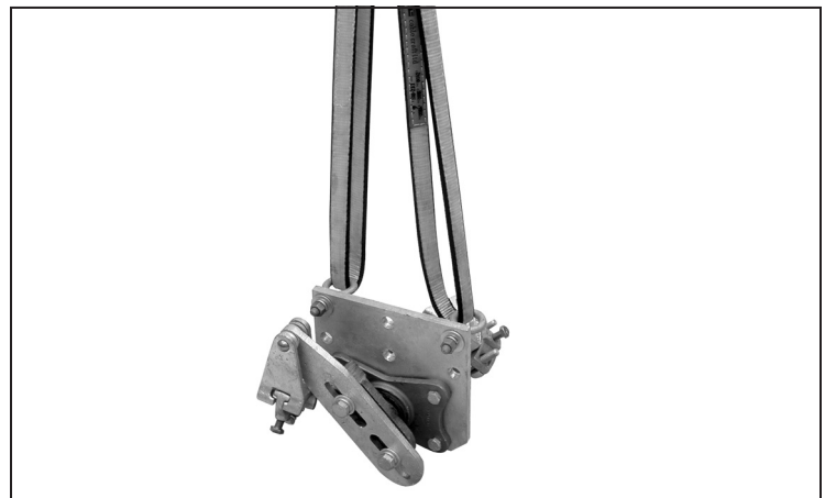
Figure 10. Hoist the outboard bearing into position.
