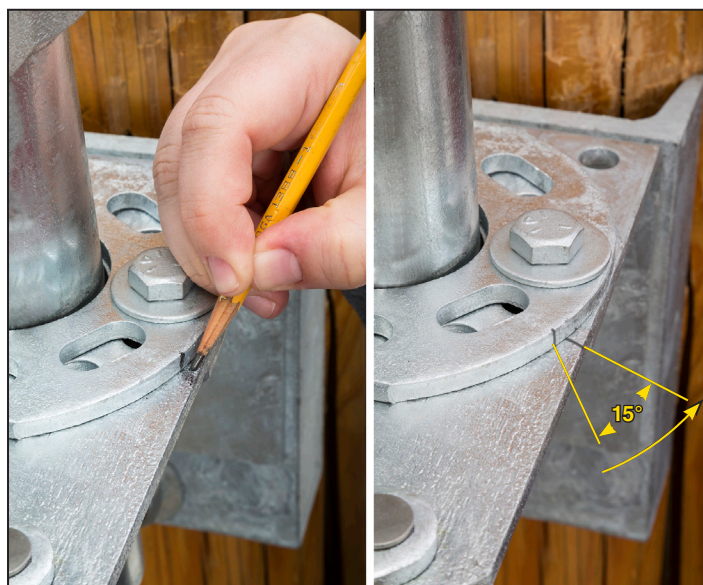
Figure 19. Mark across open and closed stop plate. Rotate the closed stop plate counterclockwise approximately 15 degrees, and then re-align the open stop plate with the mark made previously, and tighten the hardware.
