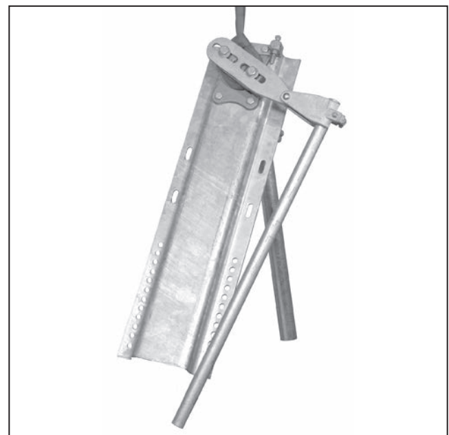
Figure 8. Hoist the outboard-bearing assembly into position.
