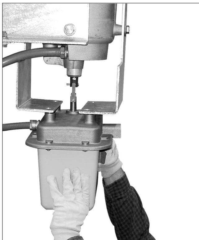
Figure 25. Disengage the operator from the operating shaft.
