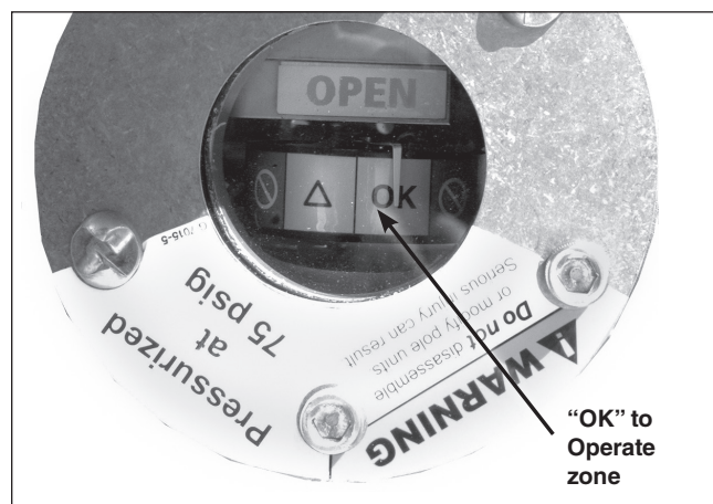
Figure 3. Indicator needle in white noting “OK” to operate zone.
