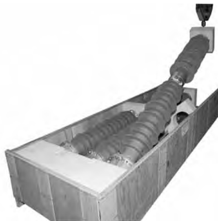
Figure 2. Pull the pole-unit carefully upward.
