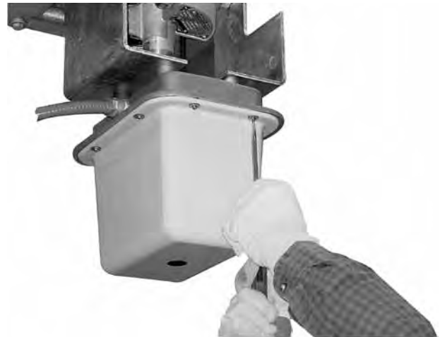
Figure 68. Remove the motor cover.
