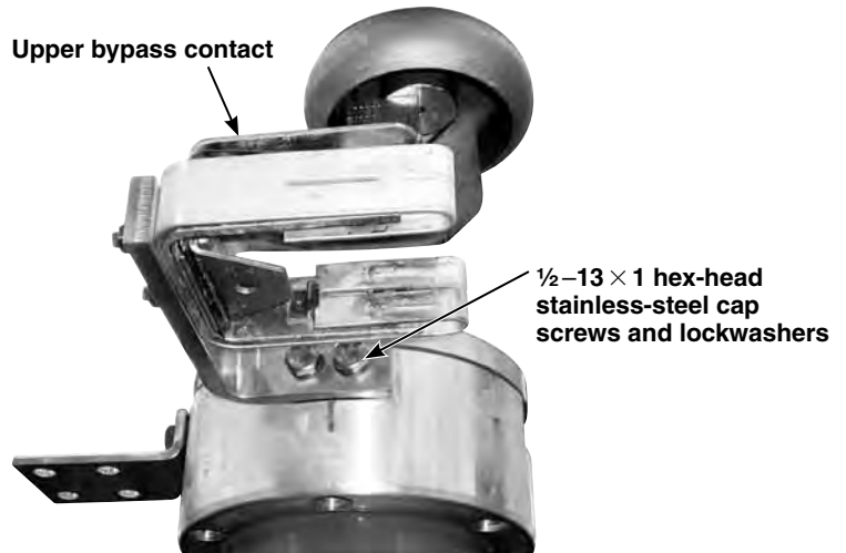
Figure 59. Attach the upper bypass contact to the pole-unit.
