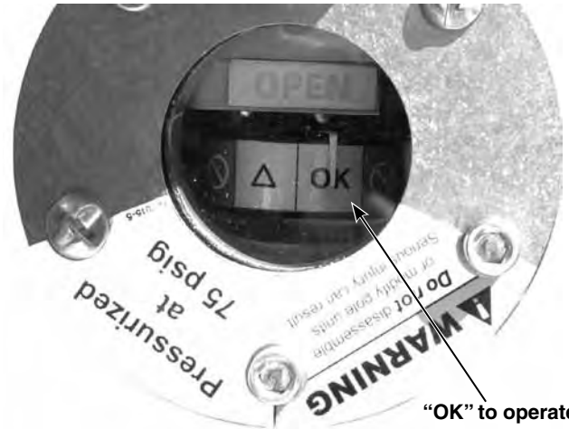
Figure 90. Gauge needle in white “OK” to operate zone.
