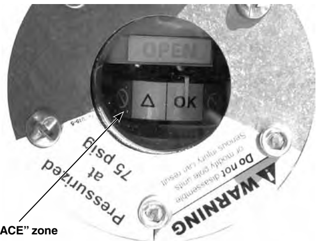
Figure 92. Gauge needle in red “REPLACE” zone.
