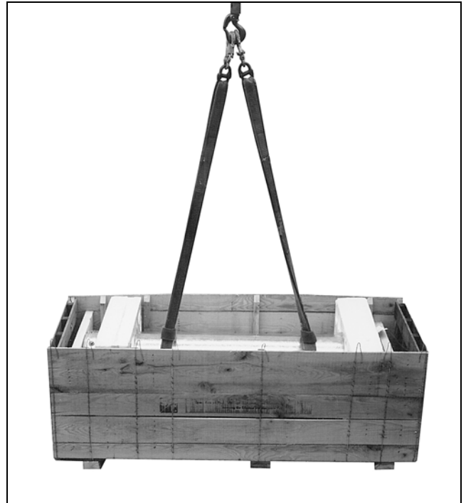
Figure 17. Removing a replacement interrupter from the shipping crate.
