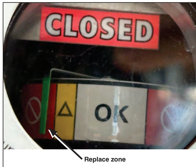
Figure 88. Gauge needle in red Replace zone.
