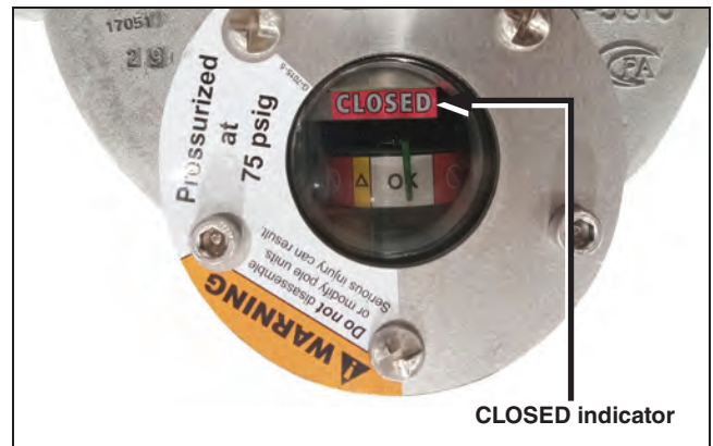
Figure 85. The interrupter is Closed and Charged. The indicator shows “CLOSED.”
