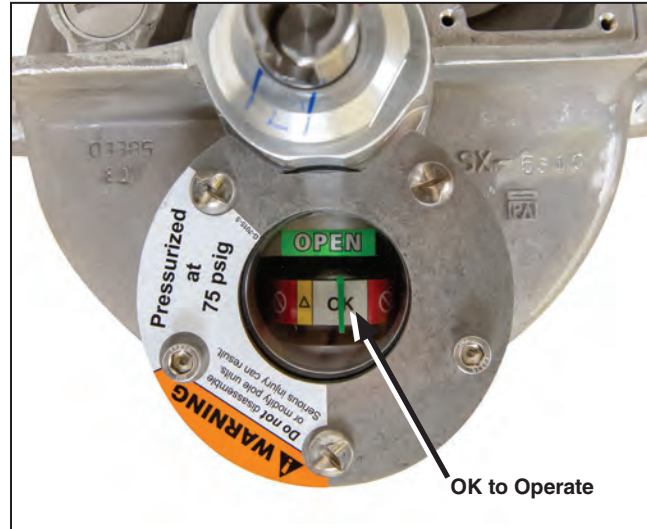
Figure 86. Gauge needle in white OK to Operate zone.
