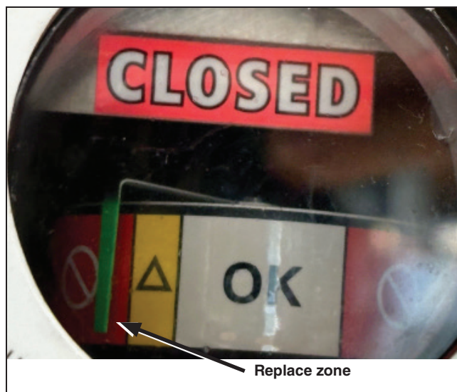
Figure 7. Gauge needle in the red Replace zone.
