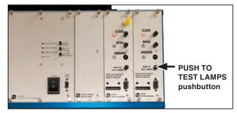
Figure 34. The PUSH TO TEST LAMPS pushbutton.
