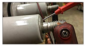
Figure 61. Take the measurement from the flat currentcarrying surface of the bushing.
