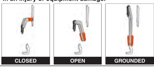
Figure 13. Confirm blade positions.
