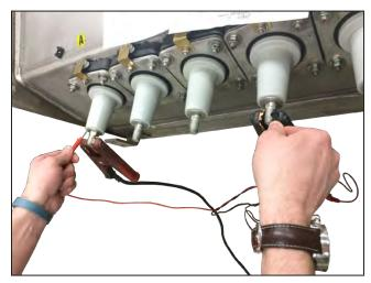
Figure 60. Connecting the resistance measuring device.
