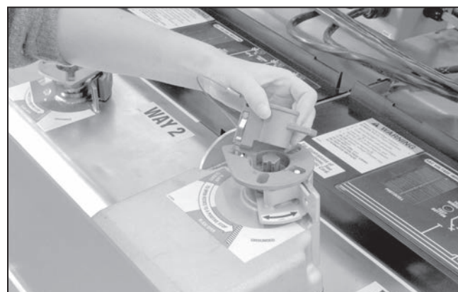
Figure 73. Remove the mechanical blocking key.
