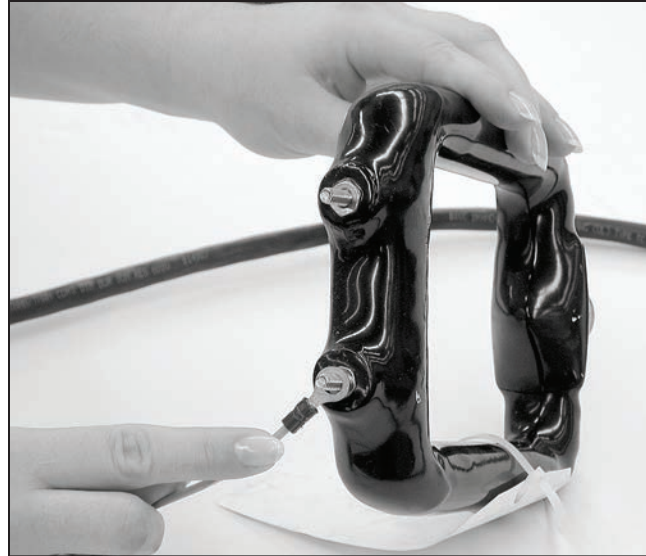
Figure 14. Attach current sensors to required wiring.
