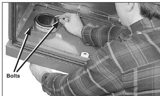
Figure 88. Install and secure the assembly through the wire pass.
