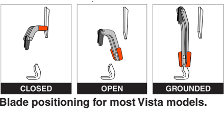
Figure 4. Confirming the load-interrupter switch or fault interrupter blade position.
