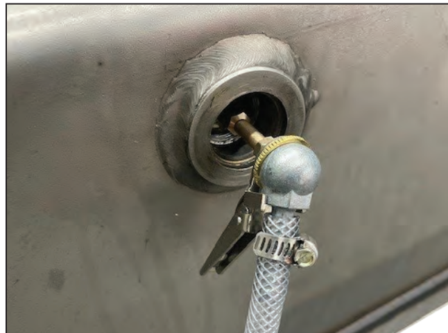
Figure 12. Connect the air chuck to the Schrader valve extender.
