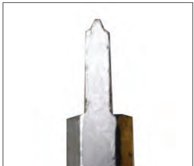
Figure 9. Fill port cover screwdriver.
