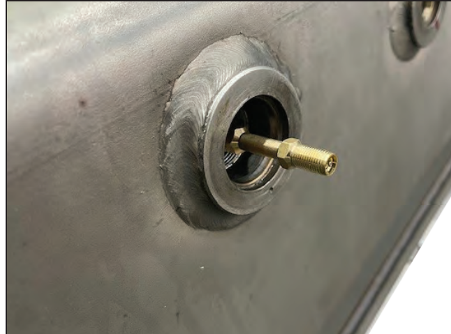
Figure 10. Thread the Schrader valve extender to the Schrader valve inside the fill port.
