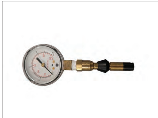
Figure 11. External pressure gauge attached to ¼-inch NPT-to-Schrader chuck adapter.
