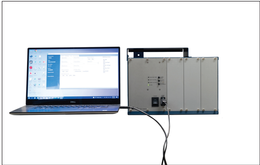
Figure 11. A USB cable connected between a PC and the Vista battery charger.
