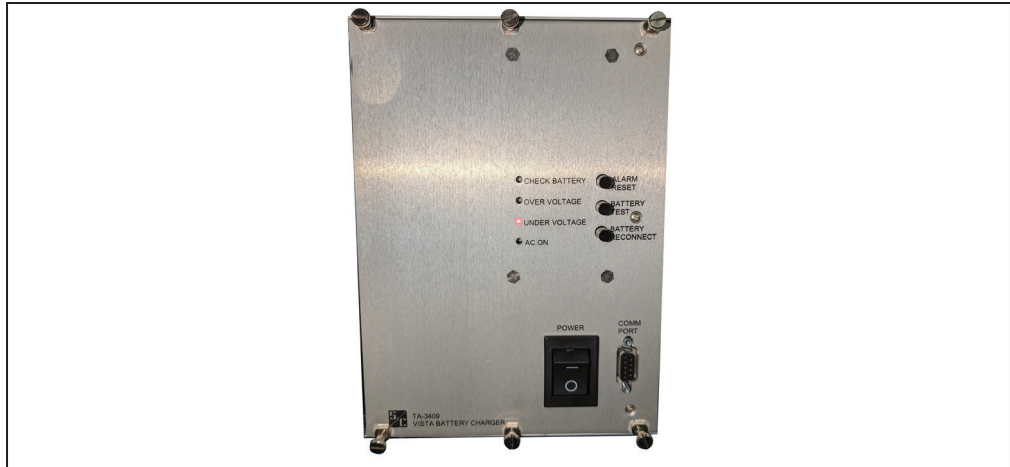
Figure 26. A battery charger with the UNDER VOLTAGE indicator illuminated.
