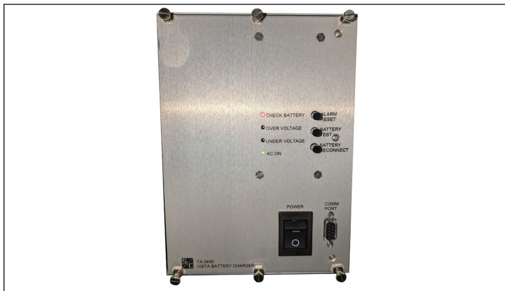
Figure 20. The Vista battery charger front panel with the CHECK BATTERY and AC ON indicators illuminated.
