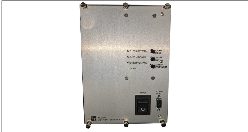
Figure 3. The Vista battery charger front panel. The AC ON indicator is illuminated.
