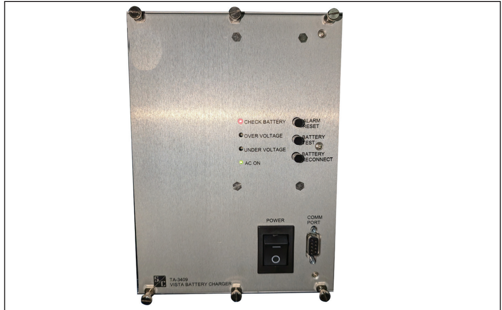
Figure 2. The Vista battery charger front panel. The CHECK BATTERY and AC ON indicators are illuminated.
