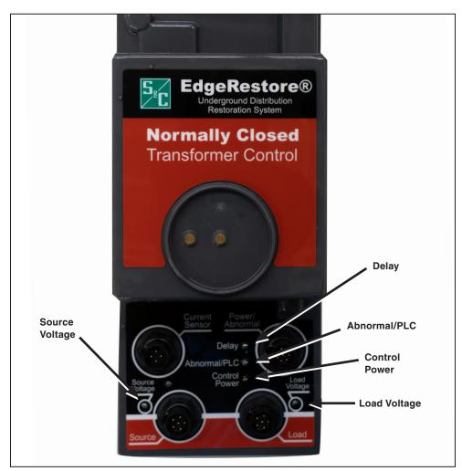
Figure 1. LED indicators on a normally closed control.
