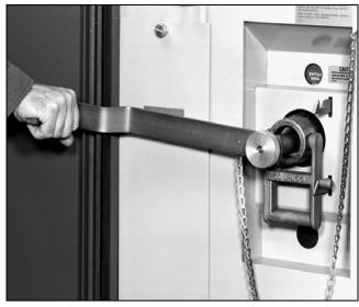
Figure 18. Dual-purpose manual handle reverse-driving the Mini-Rupter Switch and operator's quick-make quick-break mechanism to recover from a stalled condition.
