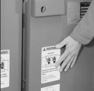
Closing door firmly push door, mechanism latches automatically when all latching points are engaged.
