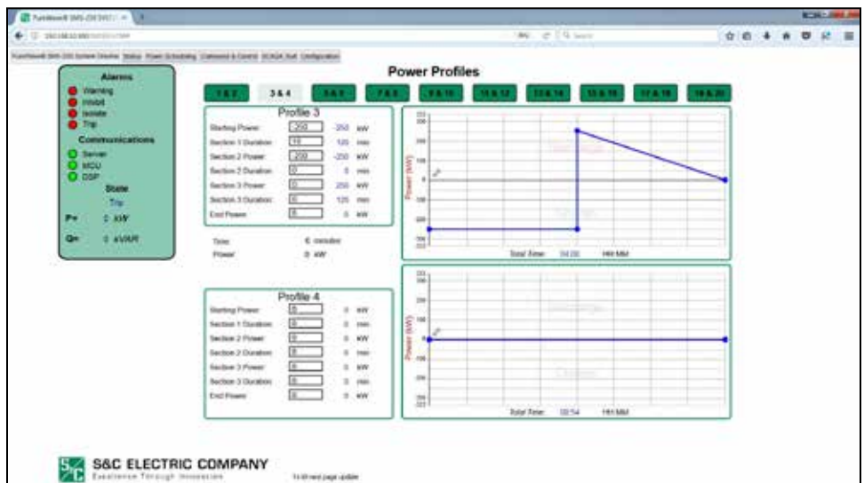
Figure 38. Power Profile screen with a Profile 3 configuration example shown within the SMS-250 HMI.
