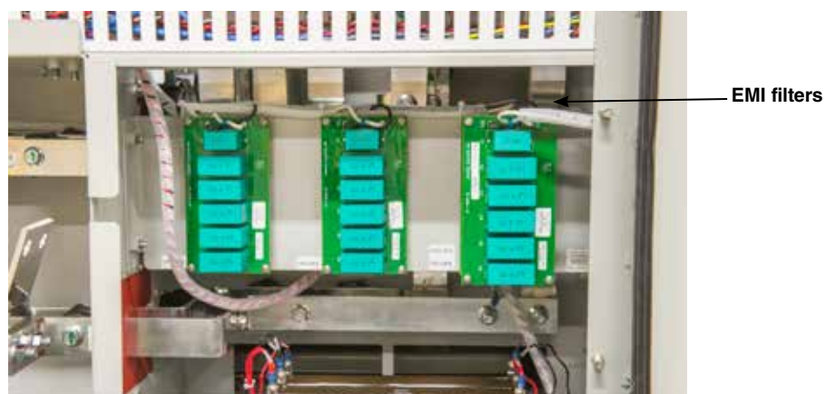
Figure 9. Location of EMI filters.
