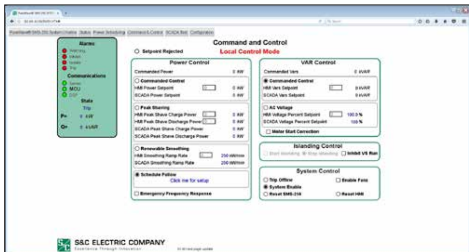
Figure 40. Command and Control screen with the Schedule Follow setting selected.
