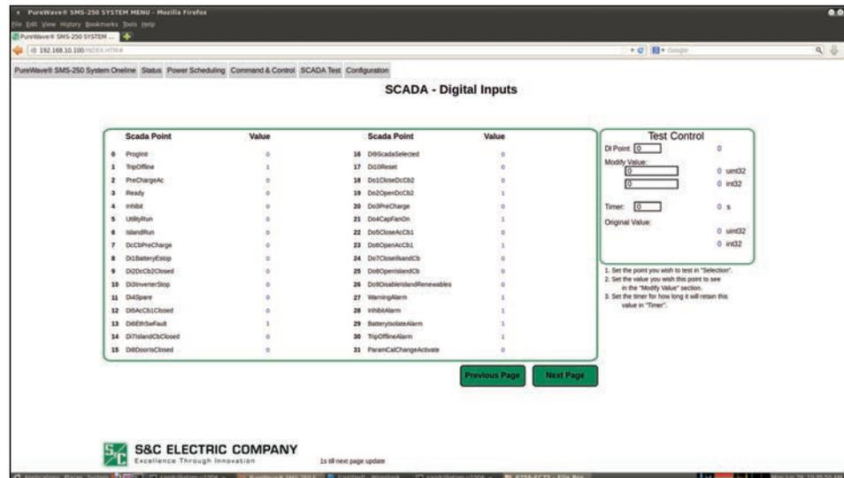
Figure 34. The SCADA–Digital Inputs screen.
