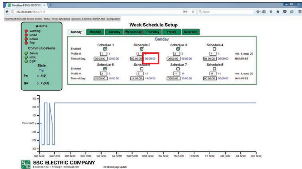
Figure 27. *Week Schedule Setup* screen with a graphical weekly profile (stored parameters indicated in red).
