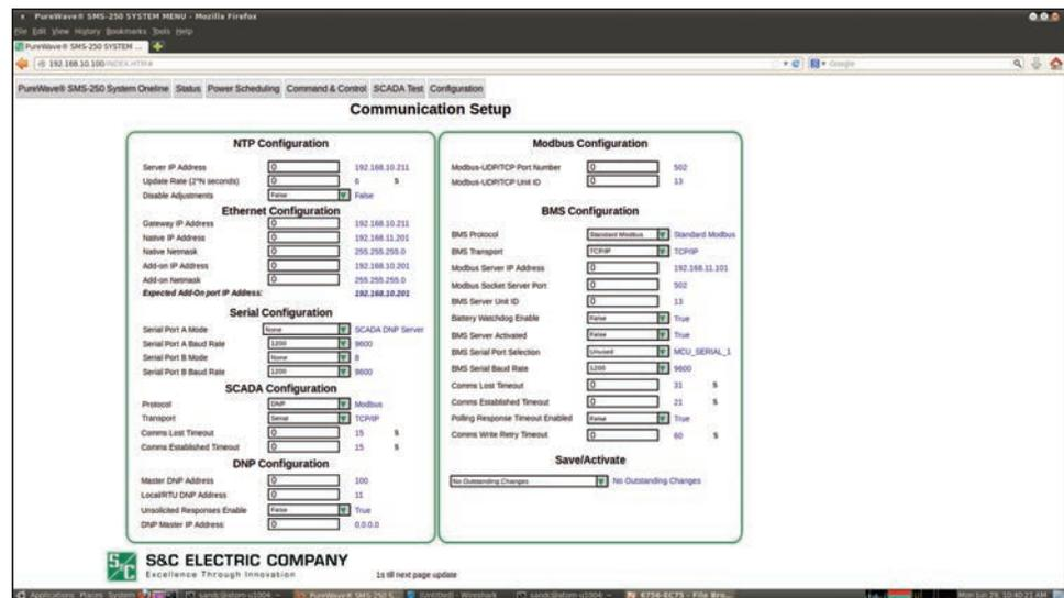
Figure 38. The *Communication Setup* screen.
