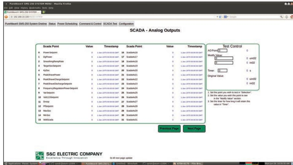
Figure 33. The SCADA–Analog Outputs screen.
