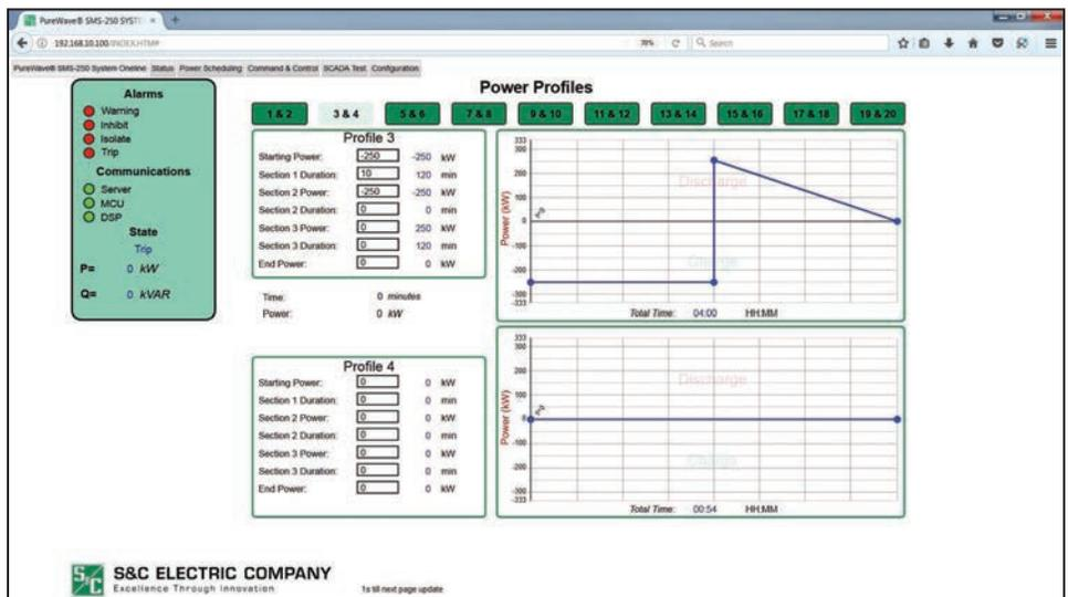
Figure 26. Power Profile screen with a Profile 3 configuration example shown within the SMS-250 HMI.
