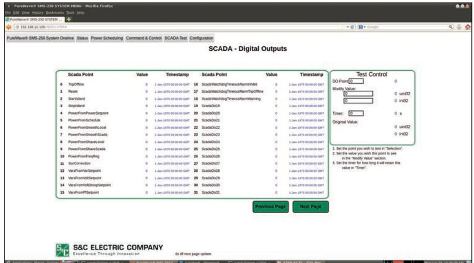
Figure 35. The SCADA–Digital Outputs screen.
