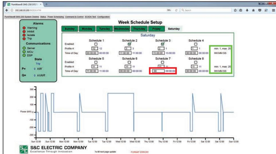
Figure 30. The Week Schedule Setup screen with no format errors.
