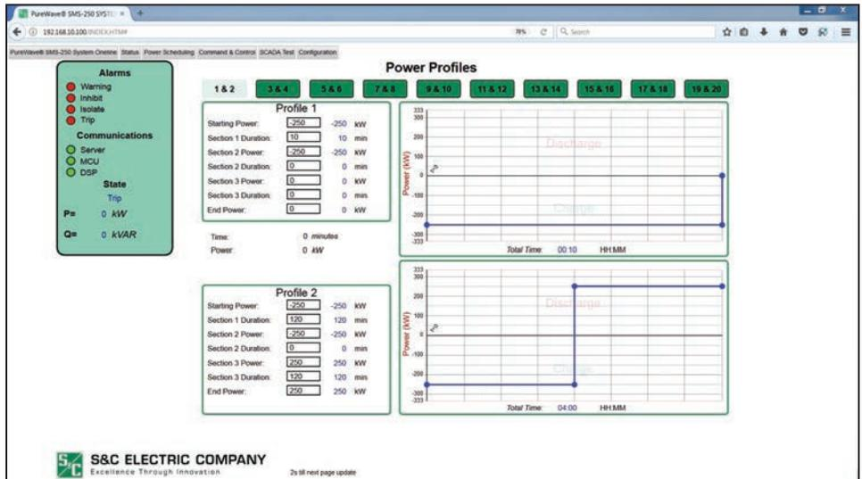
Figure 25. Power Profiles screen with Profiles 1 and 2 configuration examples shown within the SMS-250 HMI.
