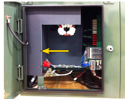
Figure 2. Shield protection from line connections (back of unit).
