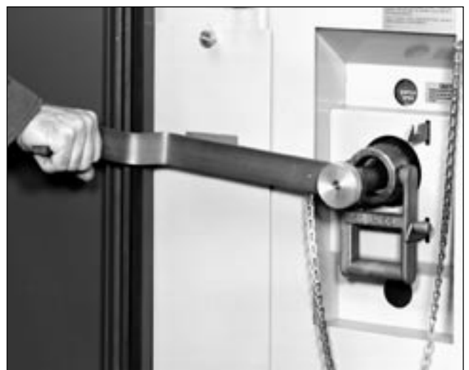
Figure 22. Dual-purpose manual handle reverse-driving the Mini-Rupter Switch and Operator's quick-make quick-break mechanism to recover from a stalled condition.
