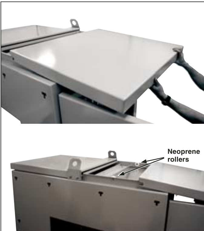
Figure 10. Sliding off roof section.
