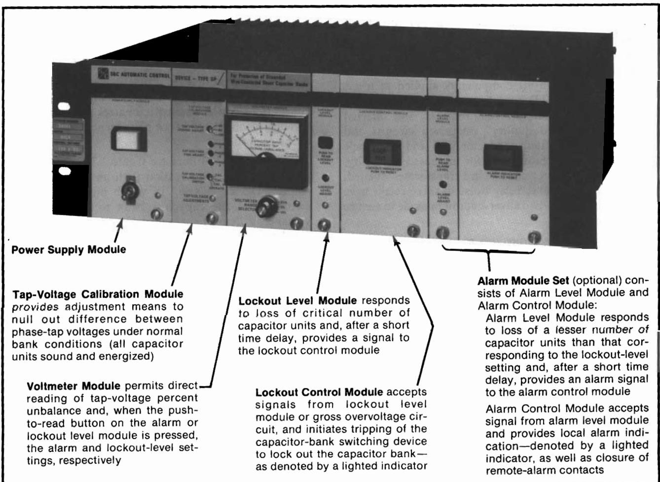
Figure 1. S&C Automatic Control Device—Type GP.
