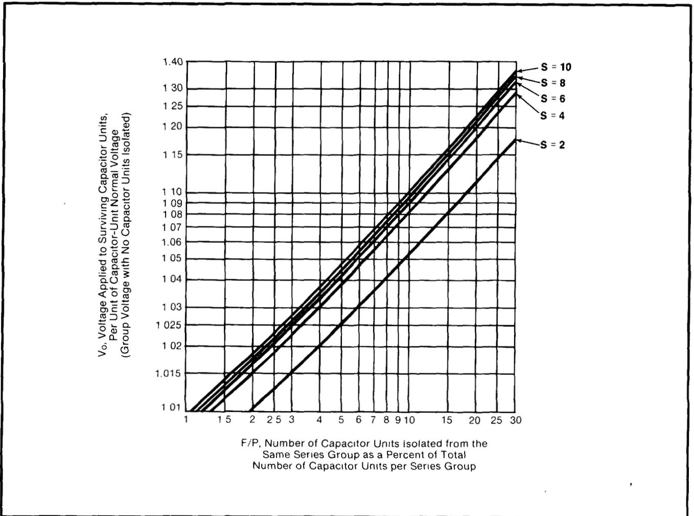
Figure 5. Per-unit voltage applied to surviving capacitor units in a series group versus percentage of capacitor units isolated from the same series group.
