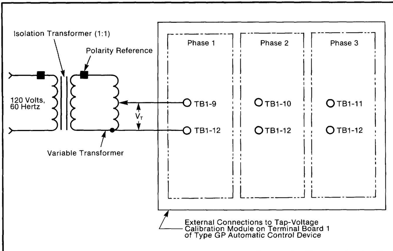
Figure 7. Connections to tap-voltage calibration module, for pre-calibrating module prior to initial energization of capacitor bank. See Step 10.
