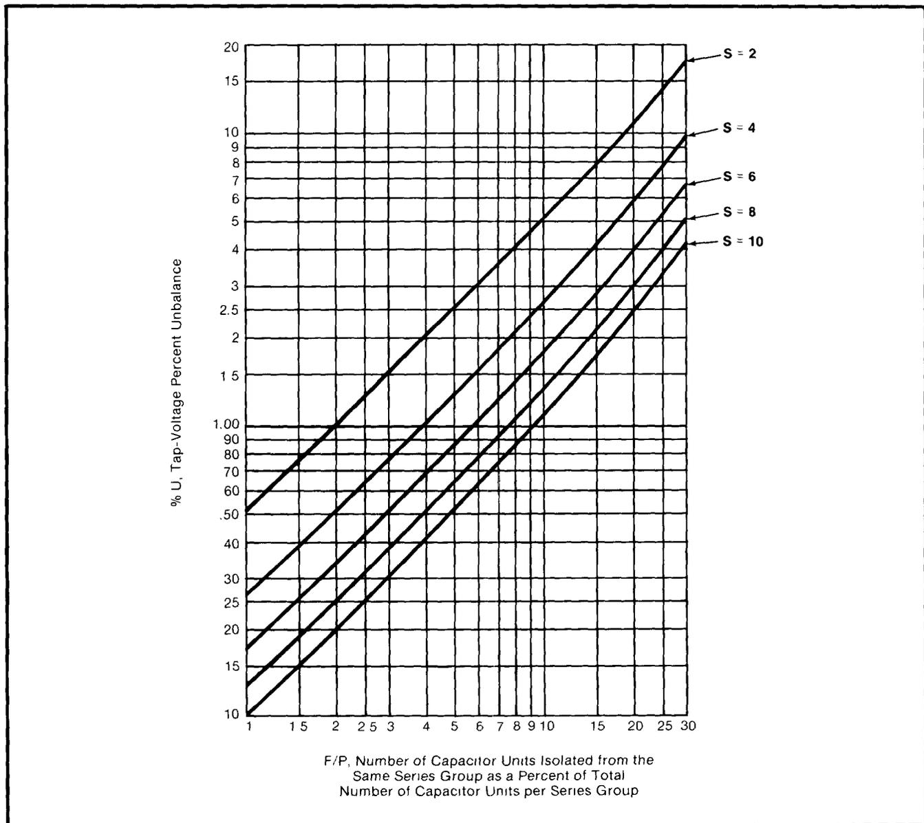
Figure 6. Tap-voltage percent unbalance versus percentage of capacitor units isolated from the same series group.
