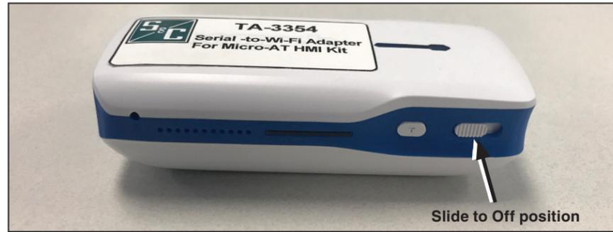
Figure 2. The adapter Power button in the Off position.
