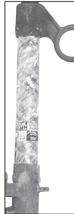
Figure 1(c). Replace: Fuse tube exhibits significant fraying.
